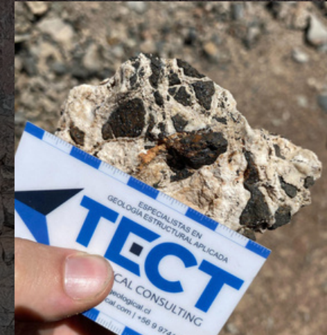
Figure 22: Mosaic-type fault breccia monomictic with clasts of magnetite [possible lenses?].
