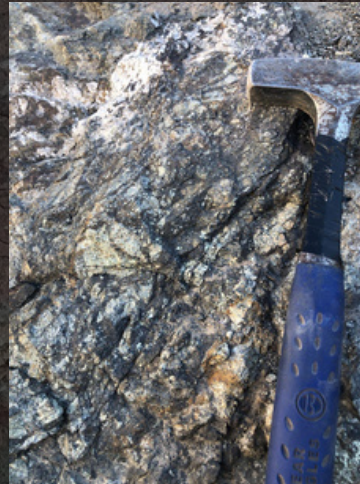
Figure 21: Monomictic breccia with fragments of diorite and matrix/cement composed of magnetite..
